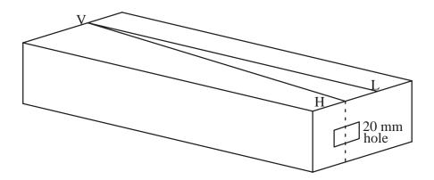
4. Center the foil over the 20 mm hole and tape it into place. Cut a vertical slit in the center of the foil, just filling the hole. Try to keep the slit very narrow—0.5 mm or less.
